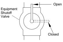
Figure 13 - Equipment Shutoff Valve
